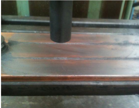
Fig. 1. Graphite Powder Filled in the Grooves of Copper Plate
